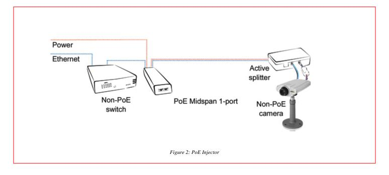
Midspans are multiport power injectors placed in series with switches. An injector is a single port midspan. Figure 2 gives an overview on how a single port midspan (injector) injects power into the Ethernet cable. The power is retrieved from the cable via a splitter box. The NCP1081 can replace the high power splitter box delivering the required high power levels.
